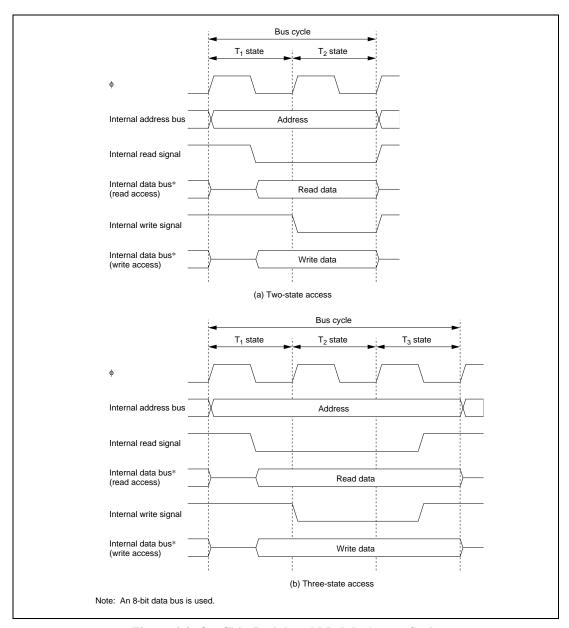
Figure 4-2. On-Chip Peripheral Module Access Cycle
