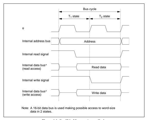
Figure 4-1. On-Chip Memory Access Cycle
