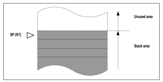
Figure 1-4. Stack Pointer
