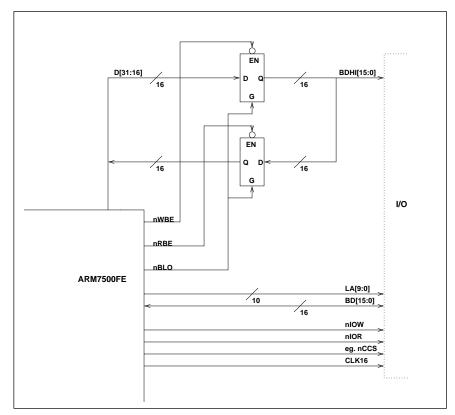
Figure D-1: 32-bit I/O interface
