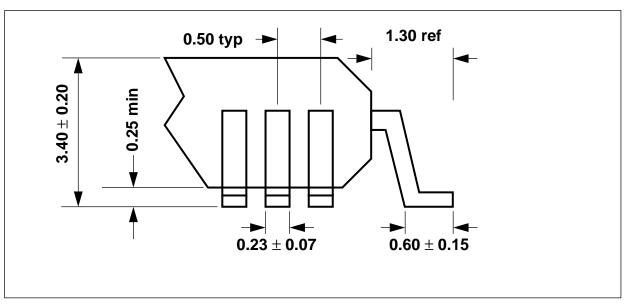
Figure 23-2: Side view of ARM7500FE chip
