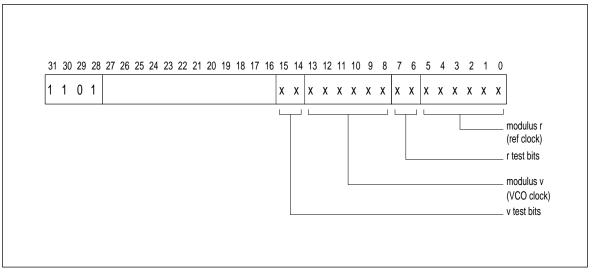
Figure E-2: Frequency Synthesizer Register
