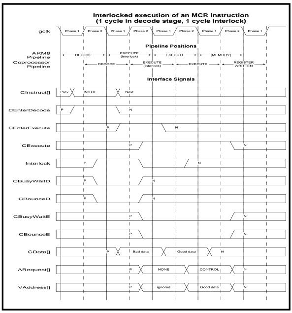
Figure 7-9: Interlocked MCR instruction operation
