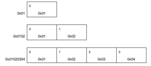
Encoding ELFDATA2MSB specifies 2's complement values, with the most significant byte at the lowest address.
